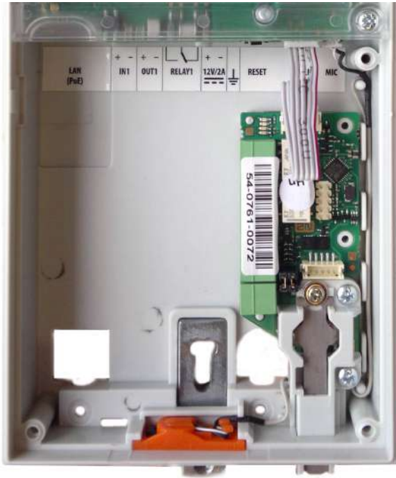
Tamper Switch Mounting
